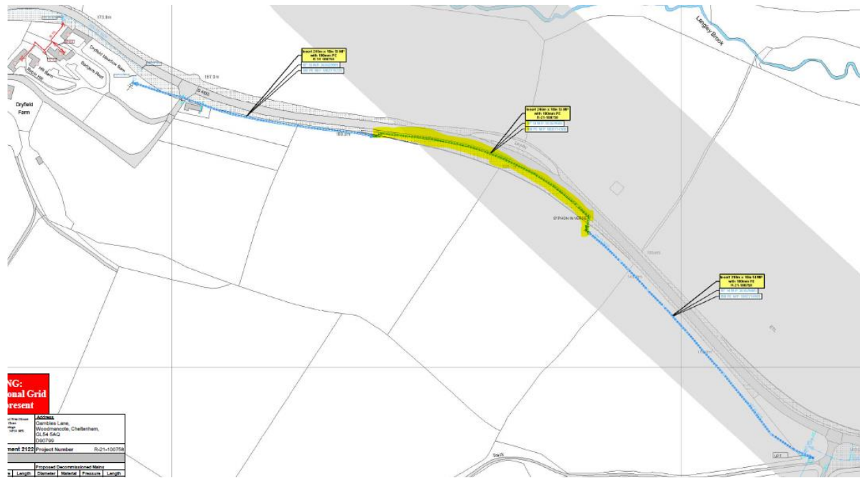
Figure 5: Shows the pipe to be replaced highlighted in yellow.
