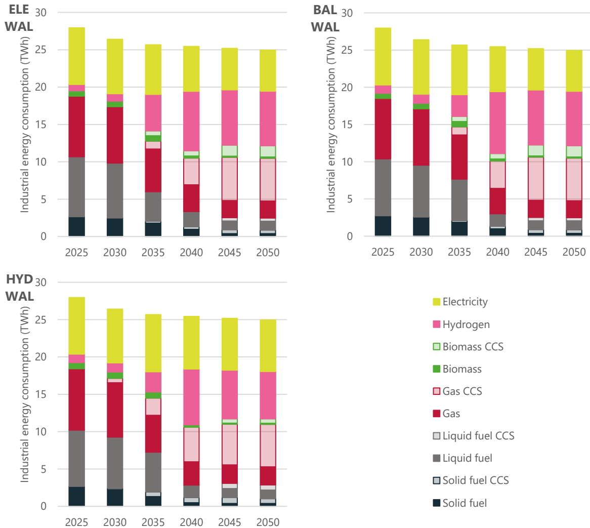
Figure 12: Industrial energy consumption broken down by energy vector in ELE, BAL and HYD scenarios. Light shaded areas correspond to consumption of energy vector with CCS
