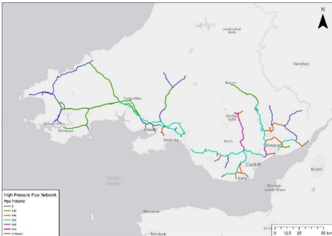
Figure 56 South Wales LTS Pipeline Material
